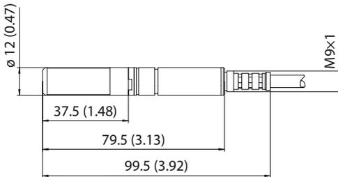
Figure 28 Dimensions in mm (inches)
