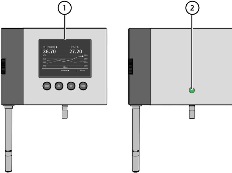
Figure 1 HMT370EX transmitter display options
