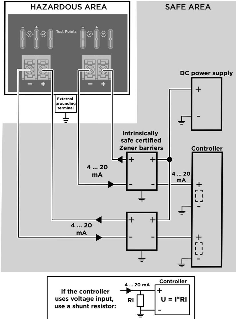
Figure 38 Wiring diagram with Zener barriers
