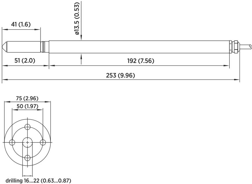
Figure 71 HMP375 probe and stainless steel installation flange. Dimensions in mm (inches).
