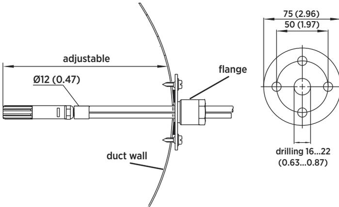
Figure 24 Left: Installation kit for duct mounting. Right: Installation flange. Aluminum or stainless steel.
