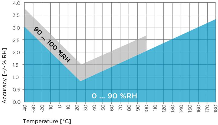
Figure 64 Humidity measurement accuracy as function of temperature
