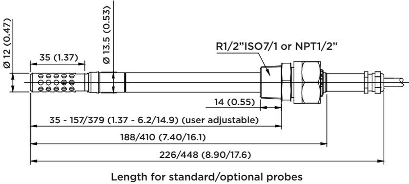
Figure 73 Dimensions in mm (inches)
