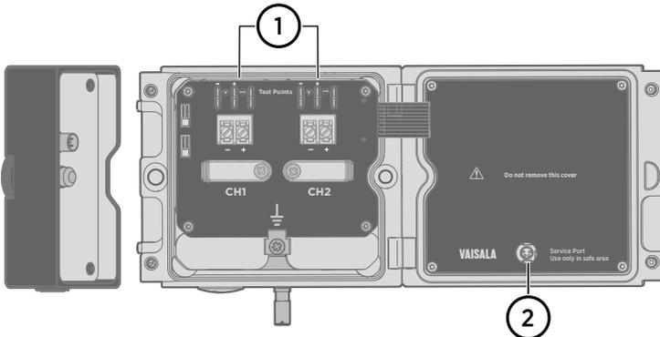
Figure 17 Location of test points and service port
