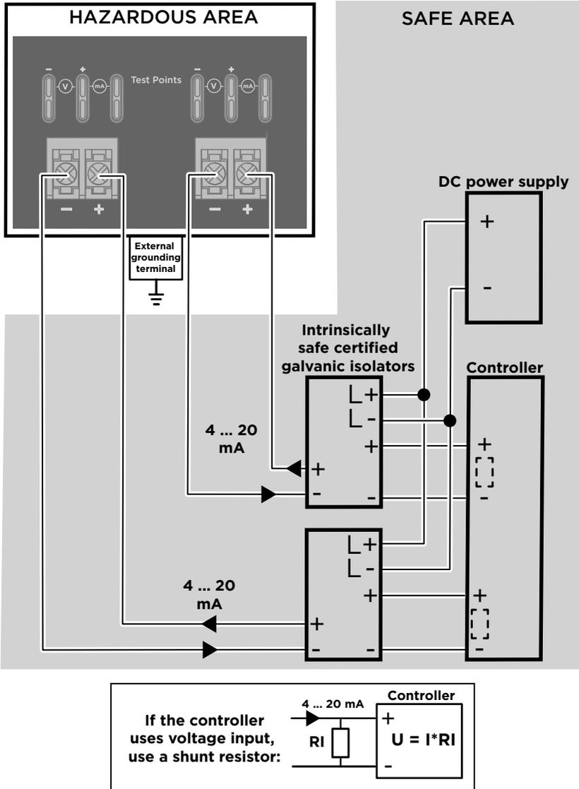
Figure 37 Wiring diagram with galvanic isolators
