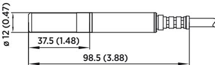
Figure 23 Dimensions in mm (inches)
