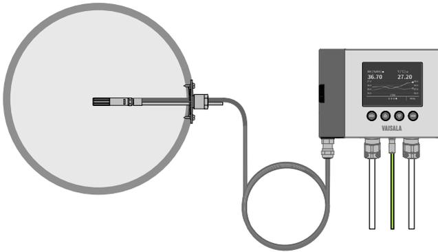
Figure 33 Duct installation example with HMP373 probe and duct installation kit
