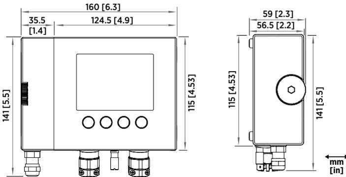
Figure 67 HMT370EX transmitter dimensions
