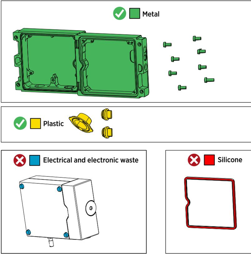
Figure 75 Recyclable and non-recyclable parts in transmitters with no display after disposing of electronics and probe
