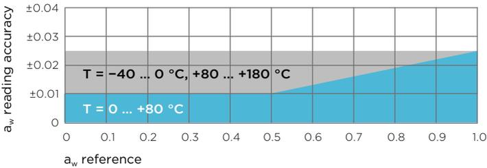
Figure 66 A<sub>w</sub> measurement accuracy
