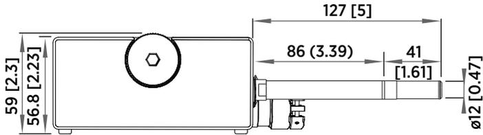
Figure 68 Dimensions in mm (inches)
