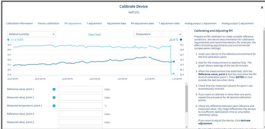
Figure 61 Insight PC software calibration view example
