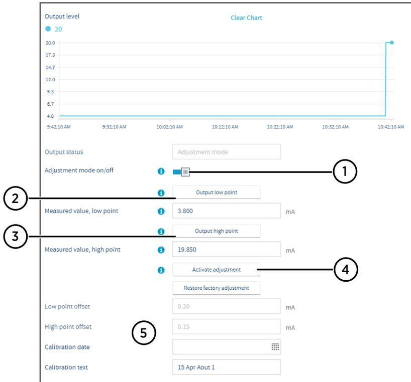
Figure 63 Analog output level adjustment in Insight PC software
