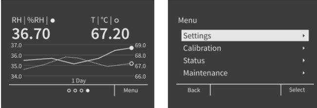
Figure 40 HMT370EX local display examples: measurement graph view and main menu screen
