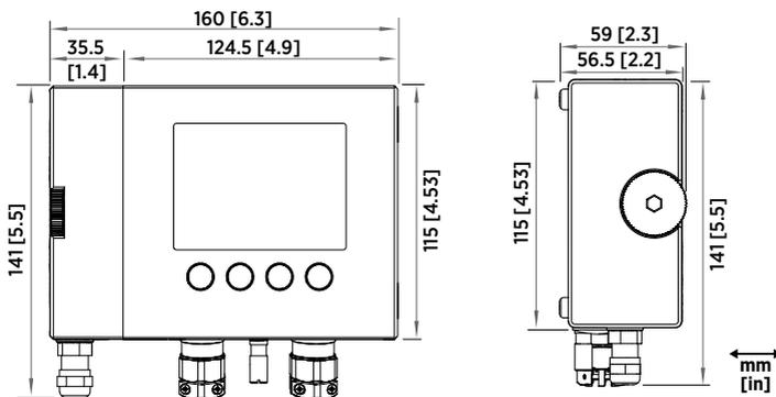
Figure 34 HMT370EX transmitter dimensions
