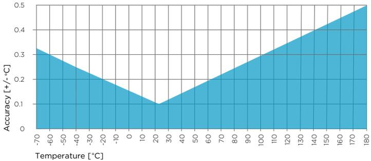
Figure 65 Temperature measurement accuracy over full range
