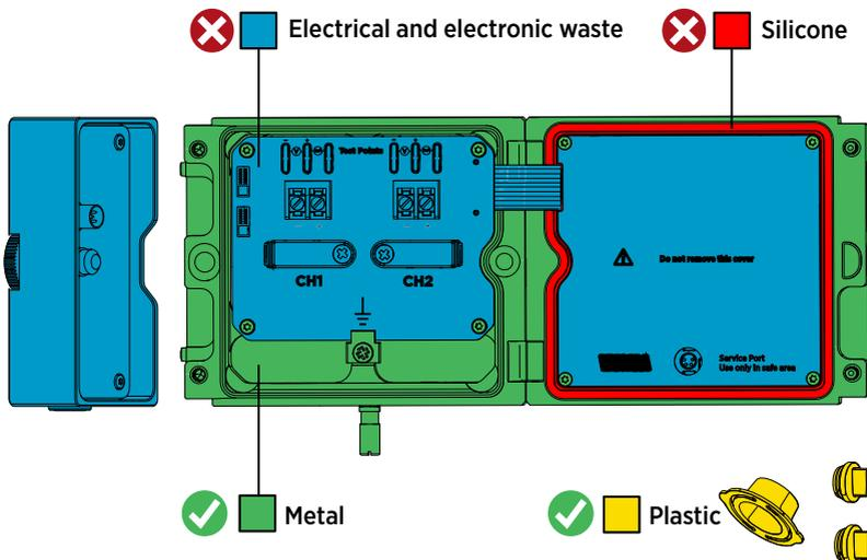
Figure 74 Recyclable and non-recyclable parts in transmitters with no display
