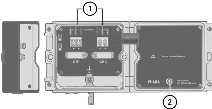
Figure 10 Location of test points and service port
