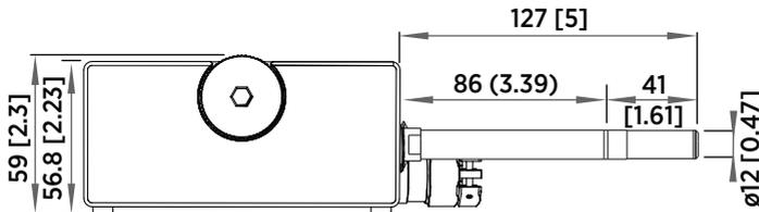
Figure 22 Dimensions in mm (inches)
