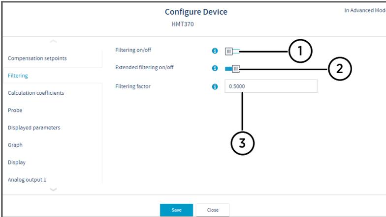
Figure 60 Filtering factor configuration in Insight PC software
