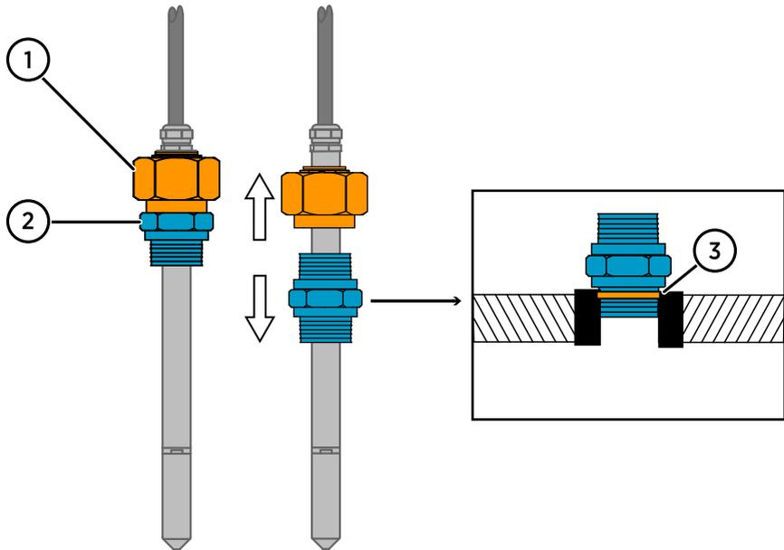
Figure 26 HMP374 fitting body and clasp nut
