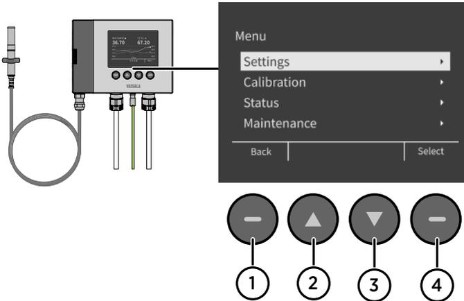
Figure 41 HMT370EX display interface buttons
