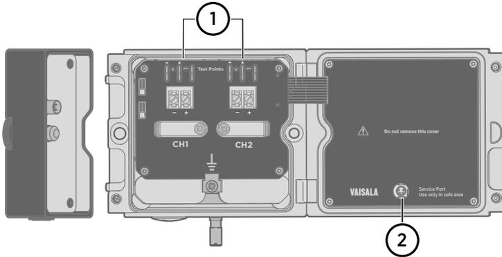
Figure 6 Location of test points and service port
