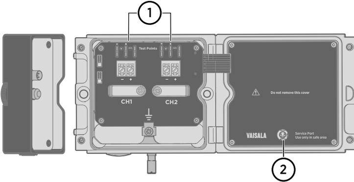
Figure 8 Location of test points and service port
