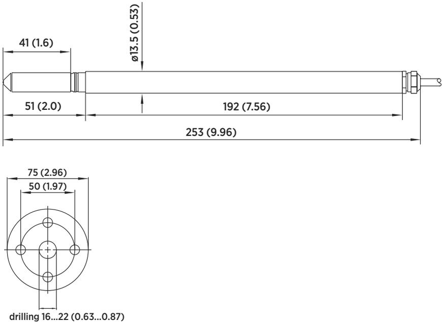
Figure 27 HMP375 probe and stainless steel installation flange. Dimensions in mm (inches).
