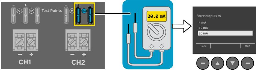
Figure 39 Multimeter test point overview
