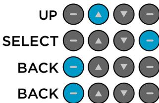
Figure 45 Display PIN code button presses
