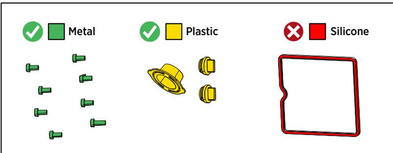
Figure 77 Recyclable and non-recyclable parts in transmitters with display after disposing of electrical and electronic waste
