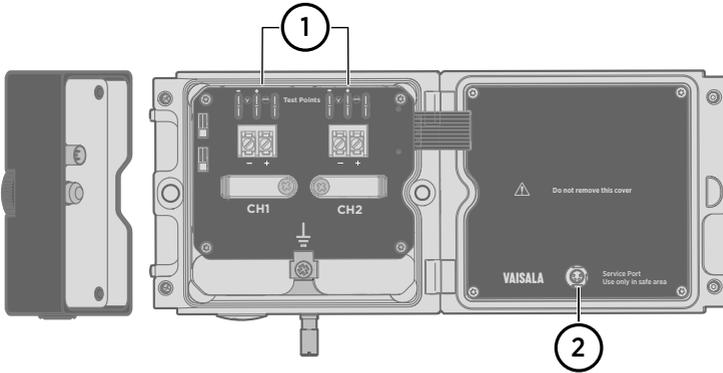
Figure 14 Location of test points and service port
