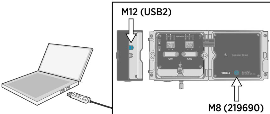
Figure 55 Connecting to Insight: probe body and transmitter service port locations
