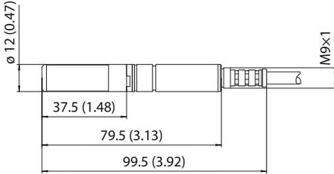
Figure 72 Dimensions in mm (inches)
