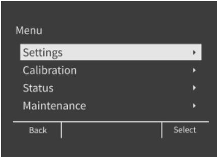
Figure 48 HMT370EX display interface main menu
