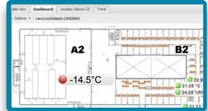
Live data showing the conditions overlaid on floor schematic
