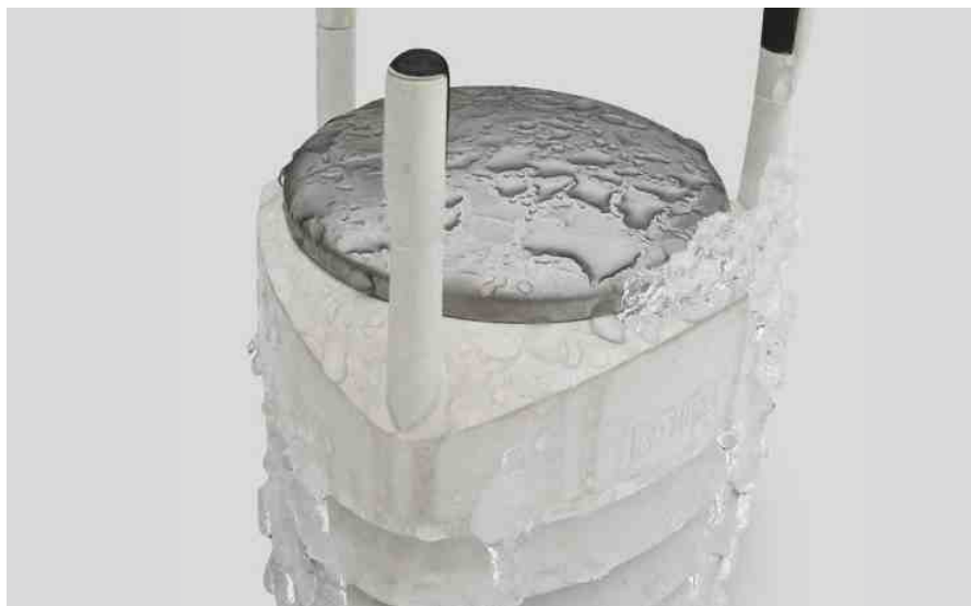
The WXT520 has an automatic control circuit that switches the heating on at low temperatures.
